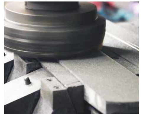
▲ The soles are milled in a number of passes to get them flat
